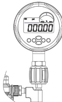
Figure 21 Connect a digital pressure gauge
