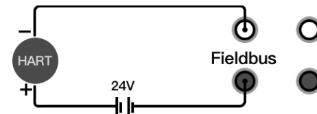
Figure 17 HART external power / internal resistance
