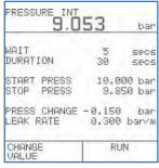
Take a 'snapshot' of the working display; all details are stored in a numbered location for later recall.
