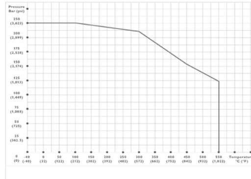
The respective max. allowable (Working) Pressure (PS) depends on the tube / pipe connection used. For further information please contact the factory.
