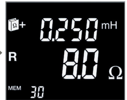
Screen 3: value of the the resistive and inductive part of the impedance measured
