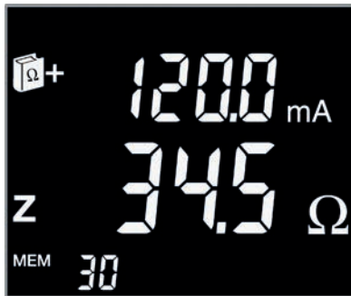
Screen 1: Impedance and leakage current
