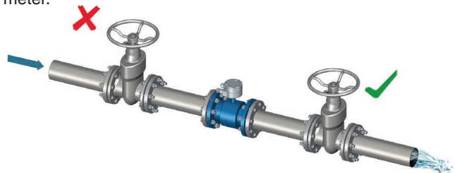
Fig. 22: Gate valves installation
