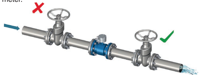
Fig. 22: Gate valves installation
