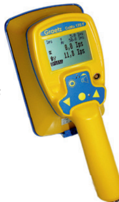
Contamination monitor CoMo-170 F for a simultaneous and selective α-, β/γ-measurement. Detector surface 170 cm².
